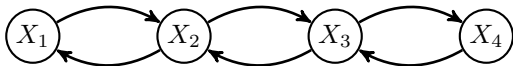
Figure 5: Graph of the structural causal model induced by the mass-spring system for D = 4 .
