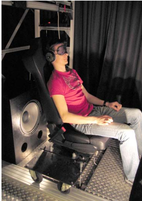
Figure 3: Laboratory setup: a participant sitting on a chair mounted on a wheeled platform connected to a wheeled footrest.
