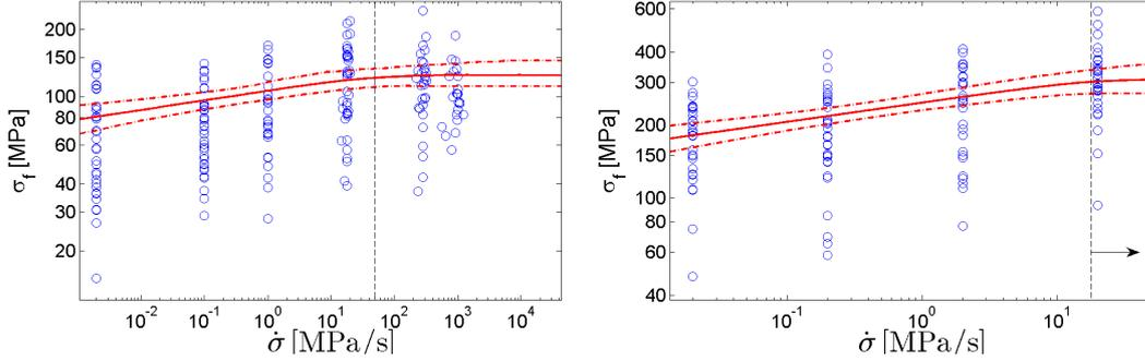
Fig. 2. Results for the data sets RB-data (left) and GS-data (right). Experimental data ( $\circ$ ) together with the median  $\sigma_o$  predicted by FBM ( $-$ ) and a 95% confidence interval ( $\cdots$ ) are shown. FBM detects where inert strengths are observed; the start of the plateau area is indicated by ( $--$ ). Note that the RB-data shows a pronounced saturation region, while for the GS-data the plateau is correctly found to lie to the right of the measurements.
