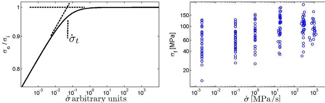
Fig. 1. The left plot shows the dependency (3) between loading rate  $\dot{\sigma}$  and characteristic failure strength  $\sigma_o$  with asymptotes (5). For materials with small Weibull parameter it can be hard to localize the plateau region from experimental data as shown by the right plot (RB-data, see Sec. 4 for details).
