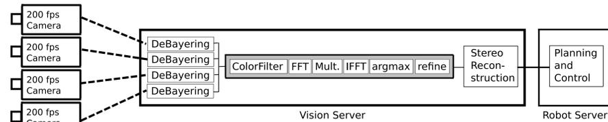
Example Setup: 200 Hz Four Camera System
