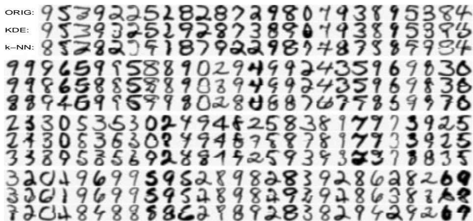
Figure 2: Errors in the digit database image reconstruction problem. Images have to be estimated using only the top half (first 8 rows of pixels) of the original image (top row) by KDE (middle row) and k -NN (bottom row). We show all the test examples on the first fold of cross validation where k -NN makes an error in estimating the correct digit whilst KDE does not (73 mistakes) and vice-versa (23 mistakes). We chose them by viewing the complete results by eye (and are thus somewhat subjective). The complete results can be found at www.conclu.de/jason/kde/kde.html .
