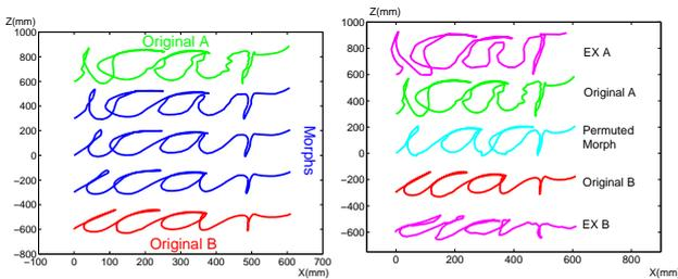
Figure 7: Left panel: Recorded pen trajectories and morphs between the original writing movements. The morphs interpolate continuously in space-time between the prototypes. Right panel: Original pen trajectories and exaggerations of the writing styles of the two actors. The middle row shows synthesis of a new word "IACR" by reassembling the movement primitives in a different sequential order.
