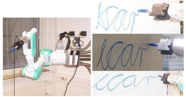
Figure 8: Left panel: The Mitsubishi PA-10 robot arm used to execute the writing movements. Right panel: Writing examples of the Originals A and B and the average morph in between (compare fig. 7).
