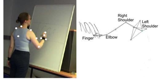
Figure 5: Left panel: Motion capturing of writing movements on a board. White dots indicate the positions of the recorded markers. Right panel: Illustration of the marker set and the trace of the finger marker during the writing of the word “ICAR”.
