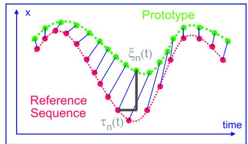
Figure 3: Illustration of the established spatio-temporal correspondence between a prototypical trajectory and a reference sequence with the correspondence vector fields  $\tau$  and  $\xi$ .
