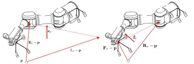
Figure 4: Illustration of the plane normals  $\mathbf{e}_r$  and  $\mathbf{f}_r$ . A virtual left shoulder  $\mathbf{L}_r$  position of the robot is defined a-priori.
