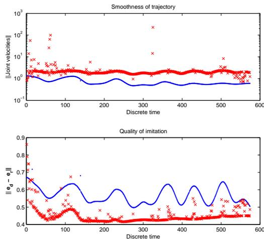
Figure 9: Joint velocities (top panel)  $\|\mathbf{q}(t_i) - \mathbf{q}(t_{i-1})\|$  and elbow norm difference (bottom panel)  $\|\mathbf{e}_d - \mathbf{e}_r\|$  as a function of time for  $\alpha = 10^{-1}$  (dots) and  $\alpha = 10^{-2}$  (crosses). One obtains continuous joint trajectories for larger  $\alpha$ .
