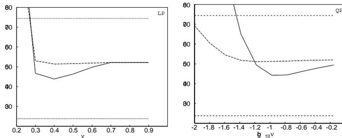
**Figure 4:** Reconstruction errors of LP and QP methods for impulse noise. The solid and dashed lines corresponds to the off-manifold and on-manifold solutions. The flat lines correspond to the least squares projection and the unrealistic setting where the correct positions of noises are given.
