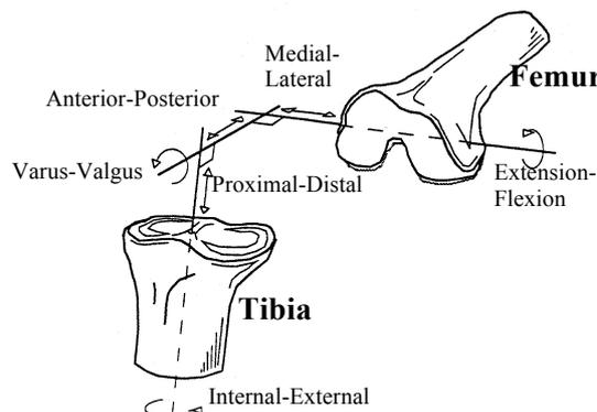
Figure 1: Knee joint rotations and translations (adapted from [5]).
