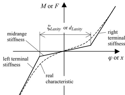
Figure 2: Elastic joint moment or force as function of rotational or translational displacement, respectively.
