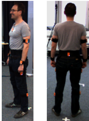
Figure 2: Sensor placement: 10 sensors are strapped to body extremities (shank, thigh, forearm, upper arm), chest and waist.
